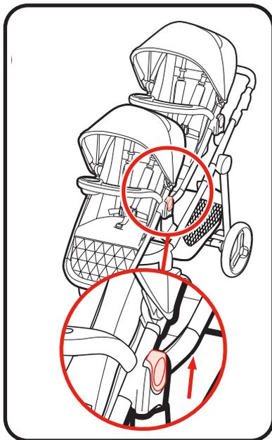
2. Push button on mount and slide lower mount into stored position. **REPEAT** on other mount.
