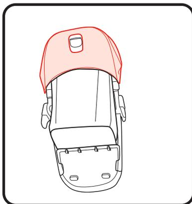
2. Flip seat and canopy over and insert 2 sets of canopy bows into mounts in seat.
