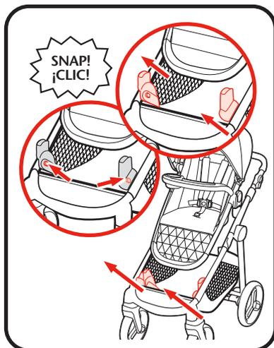
3. To attach seat, place seat on mounts as shown until they lock into place on both sides of the stroller. Seat may be placed on stroller in either direction.
