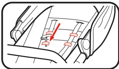
1. To adjust harness height, insert shoulder straps into desired loop.
