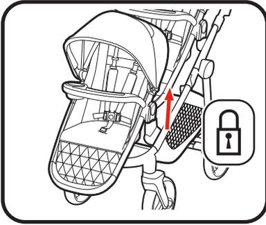
4. **CHECK** that toddler seat is securely attached to the stroller by pulling up on toddler seat.
