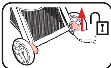
2. Push up on both brakes to unlock brakes.
