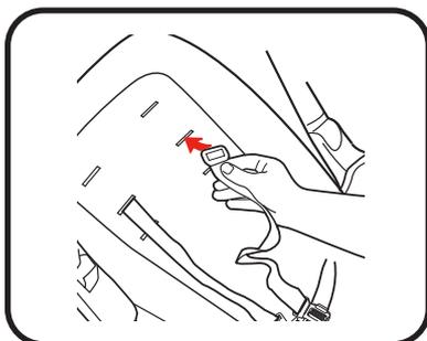
1. Push harness anchor through the front of the seat then re-insert through desired slots at the same height level. Use either shoulder harness anchor in the slots that are closest to child's shoulder height. Use slide adjuster for further adjustment.
