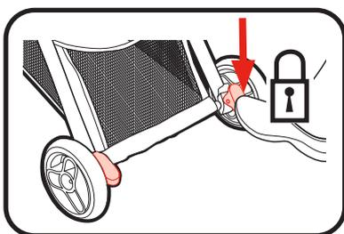
1. Push down on both brakes to lock brakes.
