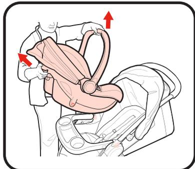
1. Recline the stroller seat back to its lowest position. Locate the 2 Click Connect™ mounts.
