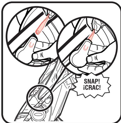
1. Insert canopy wire into the canopy mounts on each side of the stroller as shown.
