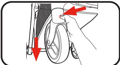
3. To remove, press button and pull wheel assembly off of stroller.
