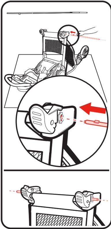
2. Insert axle rod through axle opening. Axle key must line up with key holes.
