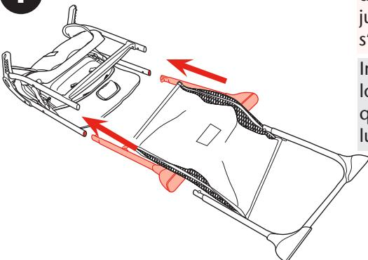
Insert "U" tube into the rear tubes until they snap into place.
