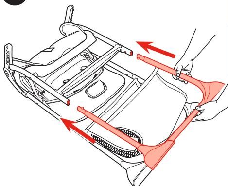
Insert "U" tube into the front leg tubes.
